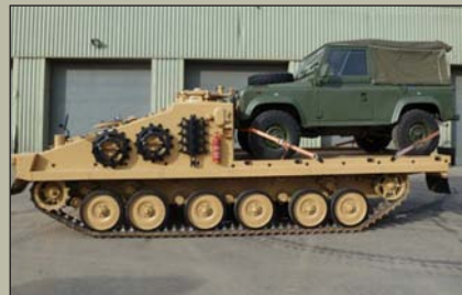
Alvis CVRT Shielder, Tracked Armoured load carrier with flat bed platform, The flat bed can adopted for a wide range of roles such as logistic carrier, bridge layer repair / recovery and towing. Built to a high specification the vehicle hull is composed of aluminium armour to protect the crew, etc, Mileage from 500, Excellent condition, Price P.O.A (20 Available)
