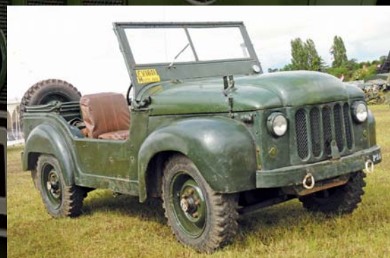
Below: also on display for the Champ Camp was an equally rare example of the Wolsley Mudlark prototype. The similarity to the Champ is clear to see, the main differences being the wider front wings and the semi-enclosed rear wheel arch panels.
