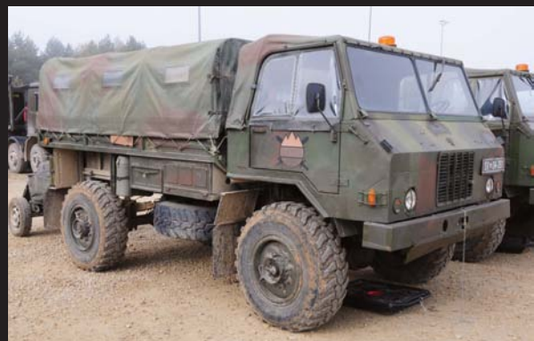
Below & bottom right: the TAM-110 light utility truck was developed in the 1980s by Tovarna Avtomobilov Maribor (TAM) to meet the requirements of the former Yugoslavian army. This truck tows a canvas covered 120mm mortar.
