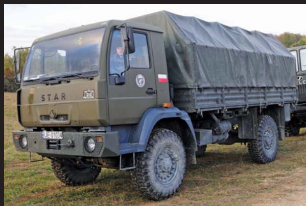
Above: the Polish Army has 650 4x4 Star 944 trucks in the inventory fielded beginning in autumn 2000. The trucks features a MAN D0824LF09 4-cylinder diesel engine developing 155hp coupled to a six-speed ZF manual gearbox and MAN two-speed transfer box.
