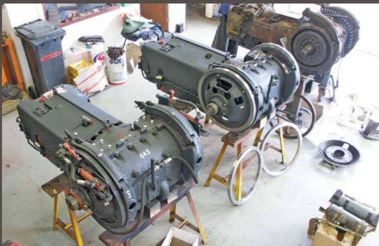
Above: three transmission units were rebuilt simultaneously, one for the Panther seen here, and two more in readiness for the other two Panthers the collection have.
